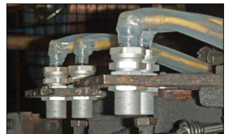
These correctly protected inductive proximity sensors will last for months or longer, safe from heat and weld cell spatter.
