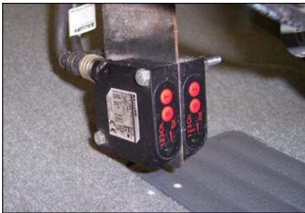
Working together, these two color sensors can exactly match and error proof color of two dissimilar floor mat materials.
