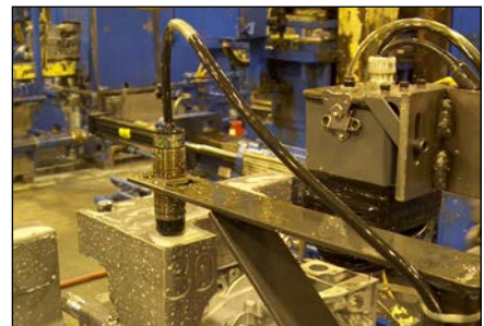
RFID sensor correctly reads build information from electronic tag through pool of cutting fluid.
