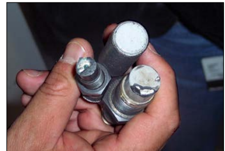
Impact has destroyed these sensors.
