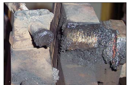
Slag build-up on sensors in weld cell.
