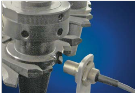
RFID read/write sensor and electronic tag error proofs automatic tool selection system.
