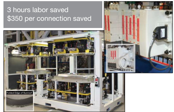
Figure 9: Kimastle Corp./Dager Systems new generation of edge folding machines – courtesy Kimastle Corp
